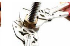
Tighten to form flange
