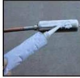
Apply heat conductive paste to condenser for better heat transfer
